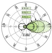
If the antennas are mounted for vertical polarization, these curves show the radiation patterns in the vertical plane.  $\[ \]$
